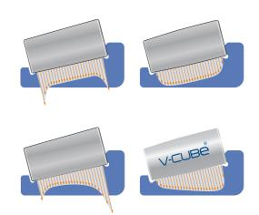
Accurate line contact between the rollers and raceways ensures optimum stress distribution at the contact points and prevents stress increases at the edges. As a result, the bearings can tolerate certain angular misalignments and give better support of moment loads.
